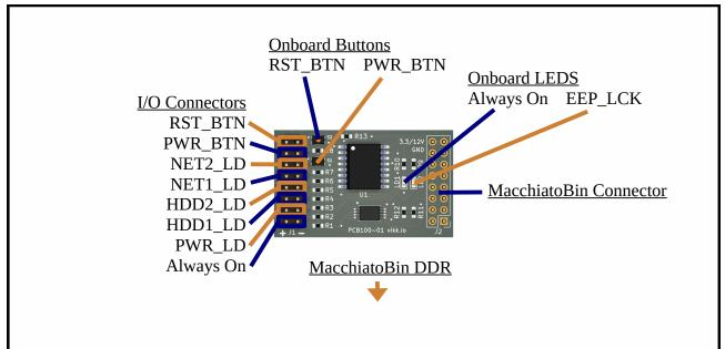
The extension board J2-header is mounted on the J12 header on the MacchiatoBin board according to pictures. The ATX case cables can then be connected to the J1-header on the extension board.
